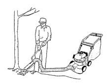
NOTE: The optional Vacuum Hose is designed for stationary vacuuming operation only.
